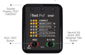
Note: The indicators will not illuminate if there is a wiring fault (missing L)
